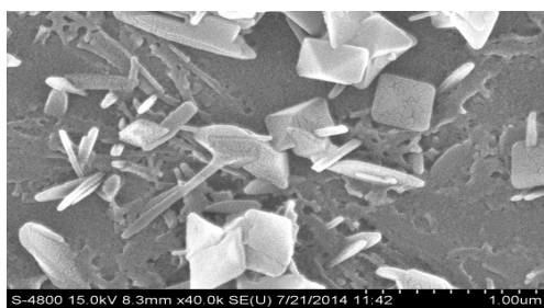
SEM micrograph of prepared \text{CoFe}_2\text{O}_4 thin film
